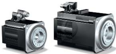
PipeDrive servo geared motor, type PY501 EZH501, one-stage gear unit with flange mount, hollow shaft, convection cooled.
